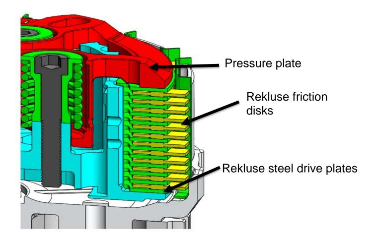
6.Install the pressure plate springs, followed by the screw sleeves and socket head cap screws (5 or 6 depending on the bike). If using two different spring colors, be sure to alternate the springs by color in every other pocket.
