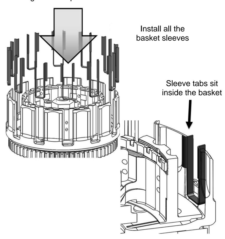
**Note:** If the basket sleeves fall forward while installing the clutch pack, us a pick to push them back into place. When seated in the basket, the sleeves may stick above or below flush with the top of the basket depending on the bike model. This is normal.
